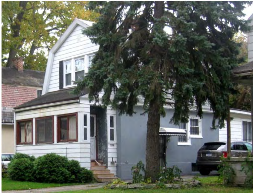
1505 W. Dartmouth St. Non-original siding, enclosed porch, vinyl or metal frame windows.
