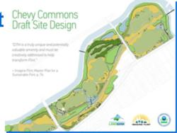
The plan calls for the site to be capped with an attractive low-maintenance natural landscape intended to minimize maintenance and storm water management costs. Details on the first three proposed phases are included in the design plan.
